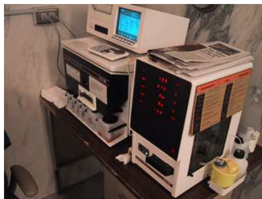
OSM3 Radiometer Cooximeter (front) and reference blood gas analyzer (rear).
